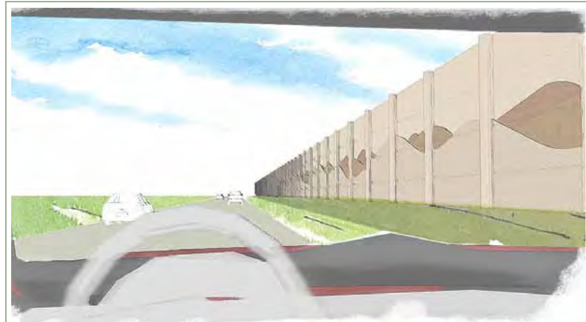
Figure 17 - Drivers' view of a sound wall concept
