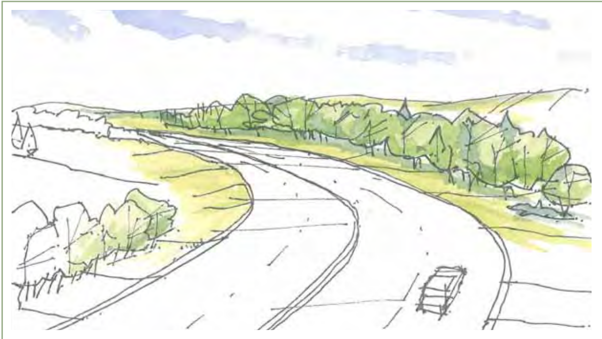
Figure 24 - Use of landscaping to delineate interstate alignment
